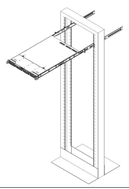
Figure 2-4. Installing the Server into a Telco Rack
